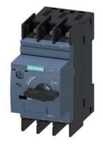
Circuit breaker size S0 for motor protection, CLASS 10 A-release 23...28 A N-release 364 A ring cable lug connection Standard switching capacity
