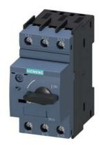
Circuit breaker size S00 for motor protection, CLASS 10 A-release 2.8...4 A N release 52 A screw terminal Standard switching capacity
