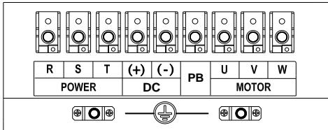
Fig.2-8 45~90kW Main Circuit Terminals
