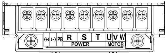
Fig.2-5 5.5~7.5kW Main Circuit Terminals
