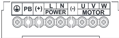
Fig.2-3 0.2~1.1kW main circuit terminals
