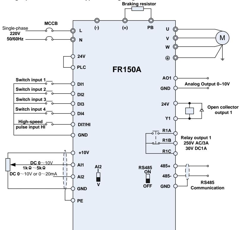
Fig.2-1 Single-phase 220V Inverter wiring diagram
