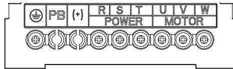
Fig.2-4 0.7~4.0kW Main Circuit Terminals
