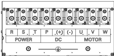
Fig.1-11 160kW Main Circuit Terminals
