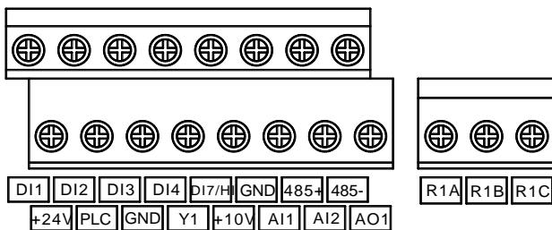
Fig.2-5 Control circuit terminals (<5.5kW)
