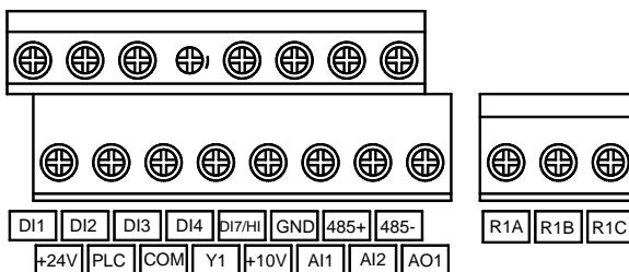
**Fig.2-6 Control circuit terminals ( $\geq 5.5kW$ )**
