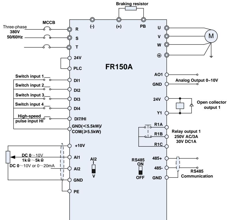
Fig.2-2 Three-phase 380V Inverter wiring diagram
