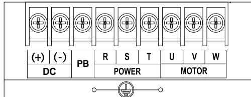
Fig.2-7 30~37kW Main Circuit Terminals
