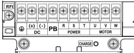
Fig.2-6 11~22kW Main Circuit Terminals
