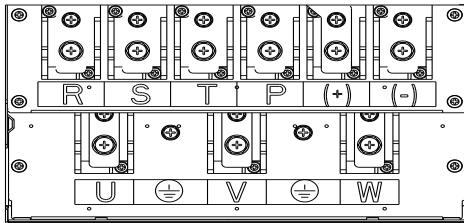
Fig.2-9 110~132kW Main Circuit Terminals
