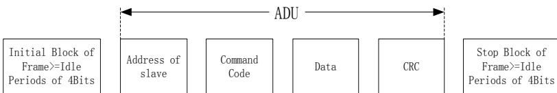
The parity in ADU (Application Data Unit) is obtained via the CRC16 parity of the 1st three Parts of ADU and switch the low bytes and high bytes. Low bytes of CRC parity go first, and high bytes of it follow in the protocol format.
