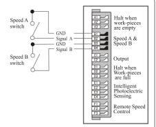
Each speed control switch has a corresponding indicator on the panel. When the controller receives an effective signal, the corresponding indicator will light up.
