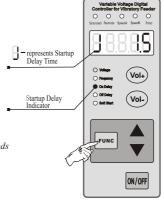
Shutdown Delay (L): The period of time the controller goes through from receiving a shutdown control signal to cutting off output.
