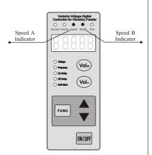
By means of speed control switches, the controller shifts to the corresponding speed. The output voltage corresponding to the speed can be adjusted by pressing (vol.) or (vol.) button. And the adjusted voltage will be stored automatically. As soon as the speed control signal is received, the controller outputs the corresponding voltage immediately.
