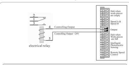
→ The controller can directly drive an electrical relay whose rated voltage is 24V and rated power lower than 4W.
